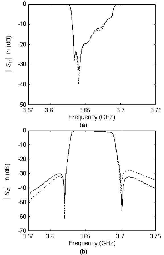
Fig. 7. Responses of the first channel of the ten-channel output multiplexer (the solid line is the ideal response and the dotted line is the EM response at the optimal design parameters). (a)  $|S_{11}|$  (in decibels). (b)  $|S_{21}|$  (in decibels).
