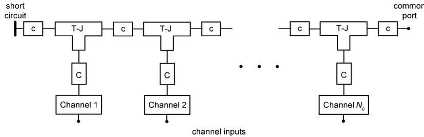
Fig. 3.  $N_c$ -channel manifold-coupled output multiplexer.
