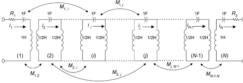
Fig. 1. Equivalent circuit of an  $N$ -coupled resonator filter.
