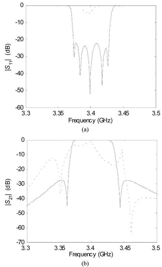
Fig. 5. Ideal responses (solid line) versus the EM responses (dotted line) by Ansoft HFSS at the initial filter parameters. (a)  $|S_{11}|$  (in decibels). (b)  $|S_{21}|$  (in decibels).
