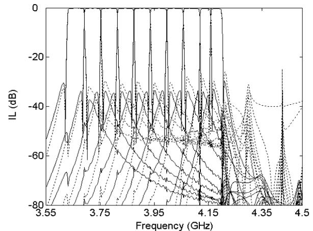
Fig. 8. Ideal response of the ten-channel DR multiplexer prototype (solid line) versus the EM response (dotted line).
