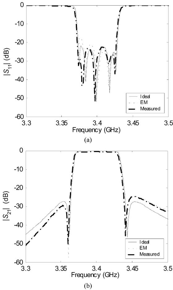
Fig. 6. Comparison between ideal responses, HFSS responses at the optimal filter parameters, and measured responses. (a)  $|S_{11}|$  (in decibels). (b)  $|S_{21}|$  (in decibels).
