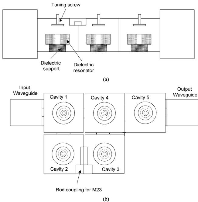
Fig. 4. Five-pole DR filter structure. (a) Side view. (b) Top view.
