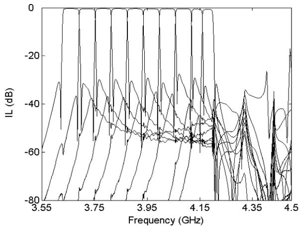
Fig. 9. Measured response of the ten-channel DR multiplexer.
